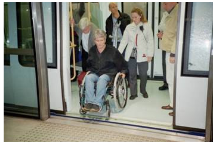
Level access metro, Copenhagen
