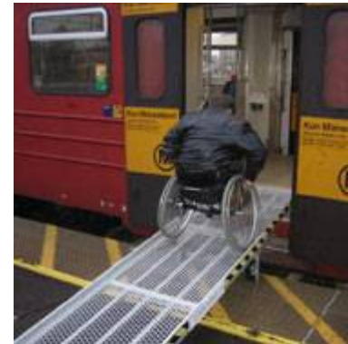
Manual ramp, Norway
